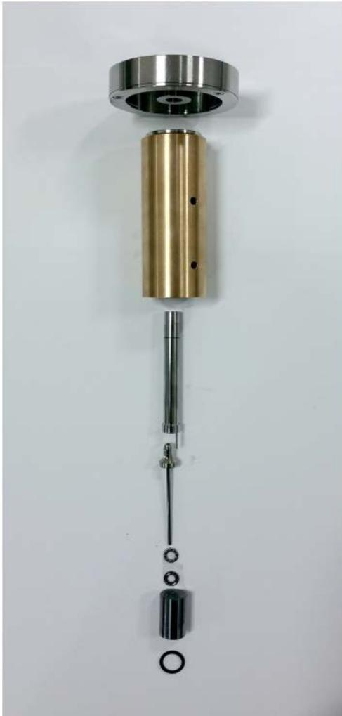
Piston assembly with small diameter = 2.25 mm
