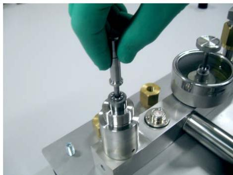
10. Mount the brass upper part and tighten it with the hook wrench. Because of the O-ring / Multi seal it is not necessary to tighten too much.
