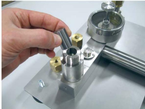
8. Turn the hand pump clockwise until oil comes out of the cylinder center hole.
